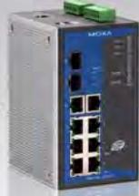
Moxa's ED5-510A-1GT2SFP-T: Managed gigabit switch with 2 SFP slots for Gigabit modules; -40 to 75C operating temp; Turbo Ring for network redundancy; supports Ethernet/IP and Modbus
